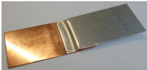
Electromagnetic pulse weld of copper to aluminium
