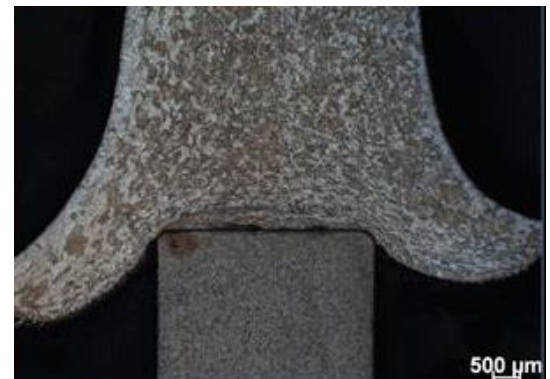
Cross section of an aluminium-steel friction weld
