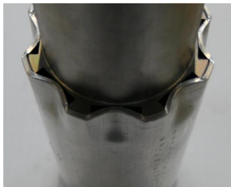
Aluminium-steel torque joint by electromagnetic pulse crimping
