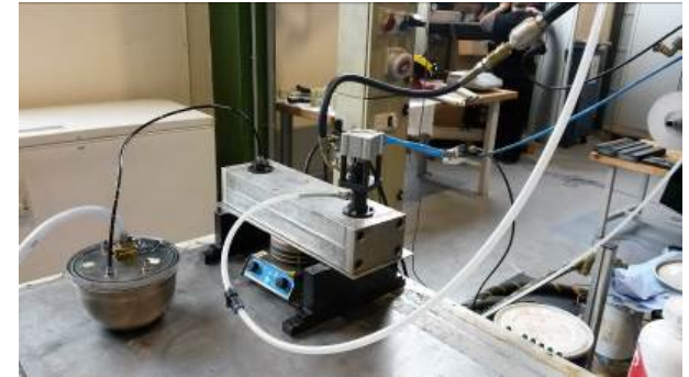
Resin injection and curing process
