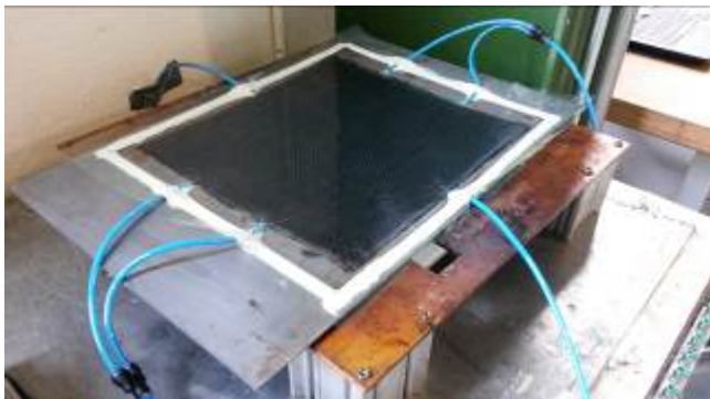
Vacuum bagging + heat
